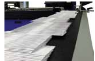
Figure 2: Creates a Continuous Separation until the next stack signal is received.
